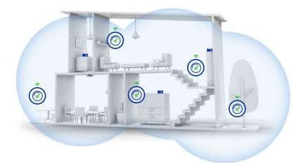
Mesh WiFi or Whole Home Mesh WiFi systems consists of a main router that connects directly to your modem, and a series of satellite modules, or nodes, placed around your house for full WiFi coverage. They are all part of a single wireless network and share the same SSID and password, unlike traditional WiFi routers.
